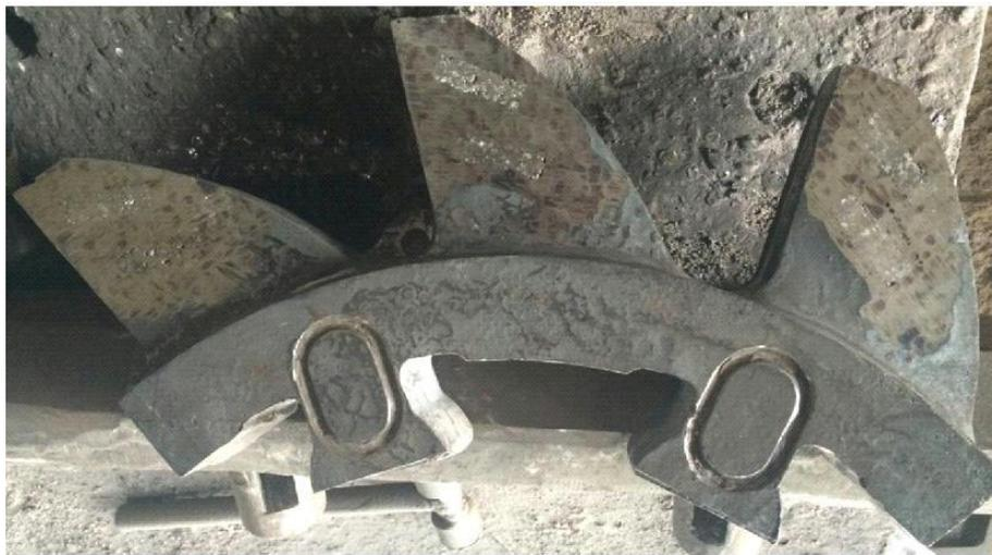
Position-1 basis material Position-2 Ceramic composites
