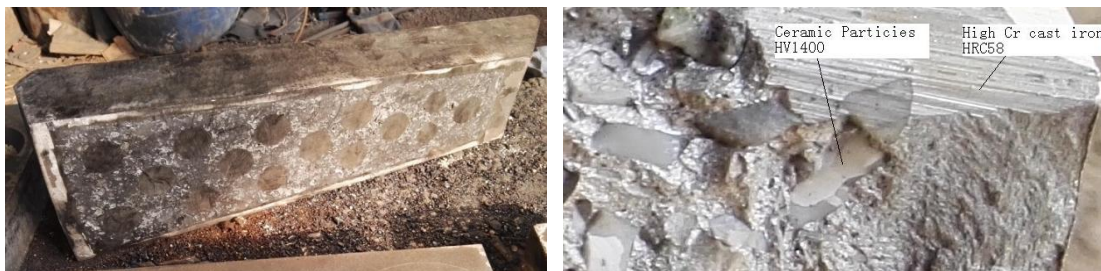
Picture 3-4 Metal Ceramic Composite Liner (HP863 Liner of High Cr cast iron +ZTA ceramic)
