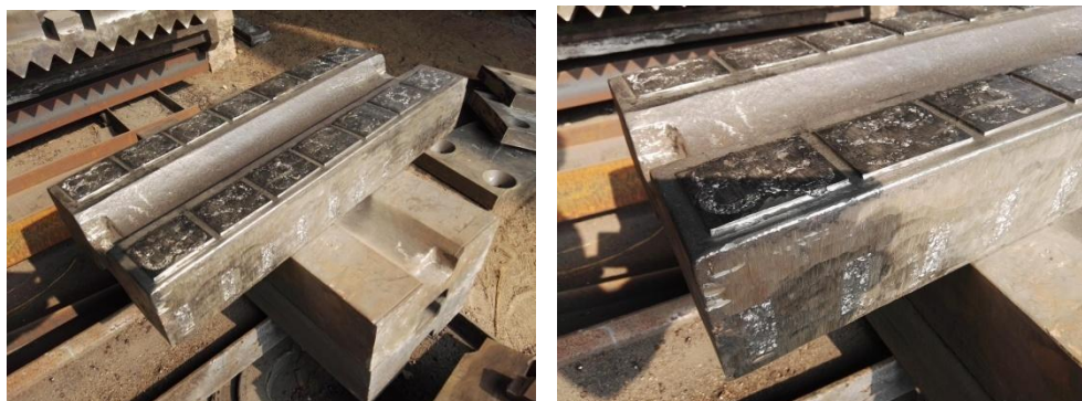
Picture 1-2 blow bar of HighCr cast Iron Ceramic composite
