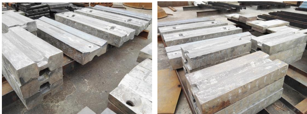
Picture 1-1 blow bar of Martensite steel ceramic composite
